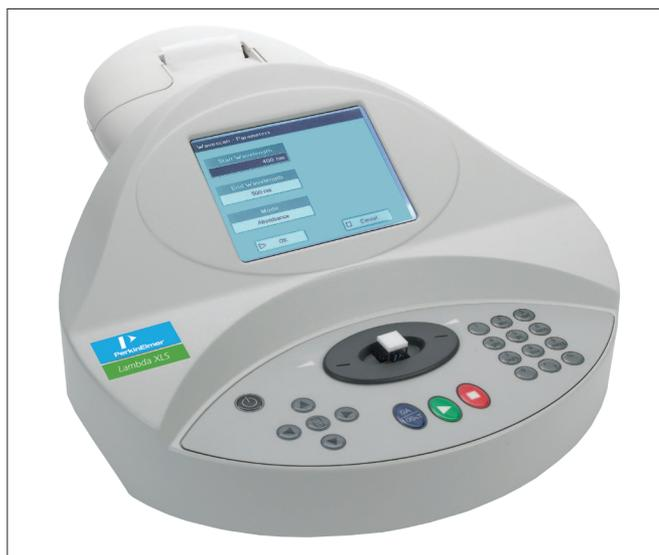
Figure 1. LAMBDA XLS UV/Vis spectrophotometer.
