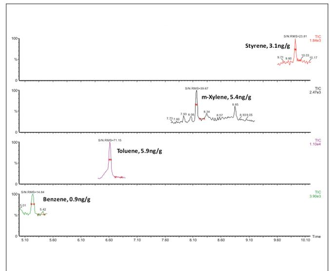
Figure 7. Chromatography of a sample containing low-levels of BTEXS with annotated signal to noise values.
