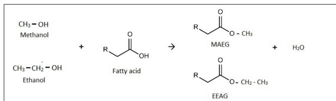
Figure 1. Esterification reaction.
